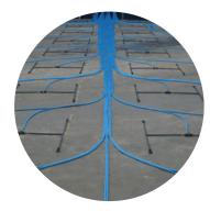
Compressed air injected in defined areas allows oxygen to be introduced
