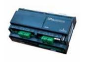
Programmable Logical Controller (PLC) iPro Genius made by Dixell, for the control of all functions. LINUX operating system, 32bit processor, 200MHz CPU, 32MB RAM, 128MB capacity.
